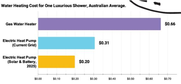
Assumes 3.93 kWh of heating required, 8 minute shower at 19L a minute. Heat Pump Coefficient Of Performance 3.77
